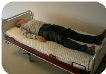
Figure 2. (a) The mattress cover with built-in sensors (b) The screen of the software you can follow the movement of the body
